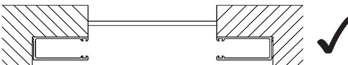
**Notice:** Do not over tighten the mounting screws. This can cause the side channel to warp, especially if the mounting surface is not flat.
