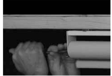
If a Wheel Adjust Bracket has been used for the Cordless Spring Drive, then turn the wheel clockwise to tighten tension and counter-clockwise to loosen tension. Repeat the necessary number of turns until the required tension is achieved.
